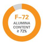
With 72% alumina content, this fiber has a soft texture conducive to textile manufacturing. Once woven and stitched, it can be fashioned into various shapes of heat-insulating seals and is also suitable for use in composite reinforcement materials.
